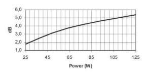
Note: These losses are calculated from a five minutes AES power test applying band limited pink noise (150-3500 Hz). The loudspeaker is free-air standing.
