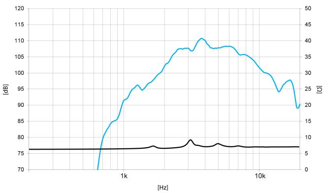
Note: On axis frequency response measured coupled to TD-164 horn in anechoic chamber, 1W / 1m
