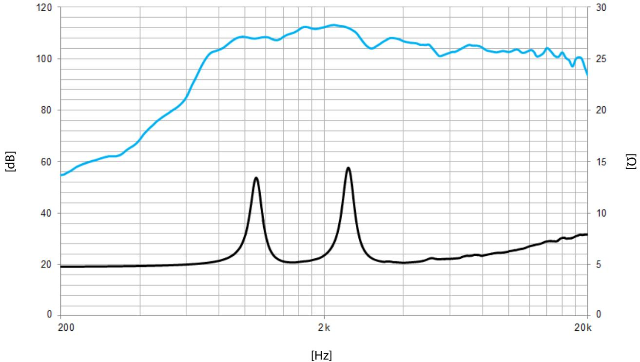
**Note:** On axis frequency response measured coupled to TD-164 horn in anechoic chamber, 1W / 1m
